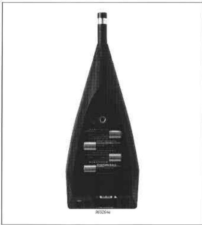
Fig.2.3 The 2237 Controller with the battery lid removed
